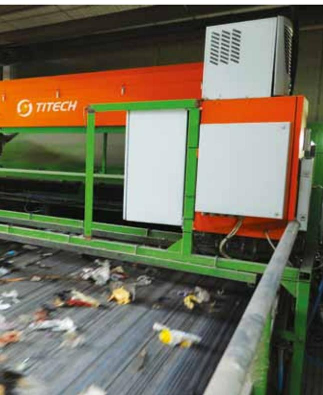
Purity levels have also improved dramatically, with sensor-based technology recovering materials of typically more than 95% purity, guaranteeing maximum revenue return.
