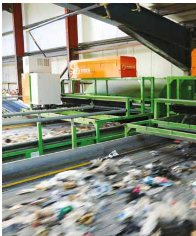
this include the use of high-resolution NIR for plastic recovery from organic fractions between 10-50mm along with the plastics and fibre from >50mm.
