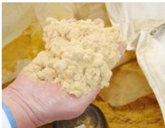
Fibre recovered from the process, in a form that can be used in MDF manufacture or other industrial applications
